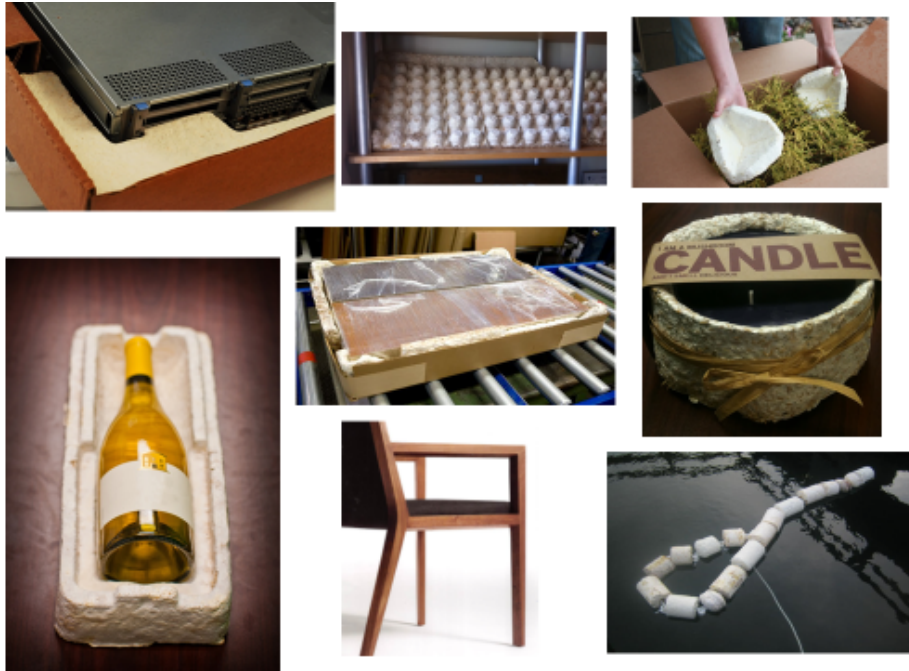
Figure 2. Various applications where the myceliated composite is currently being used or evaluated.
