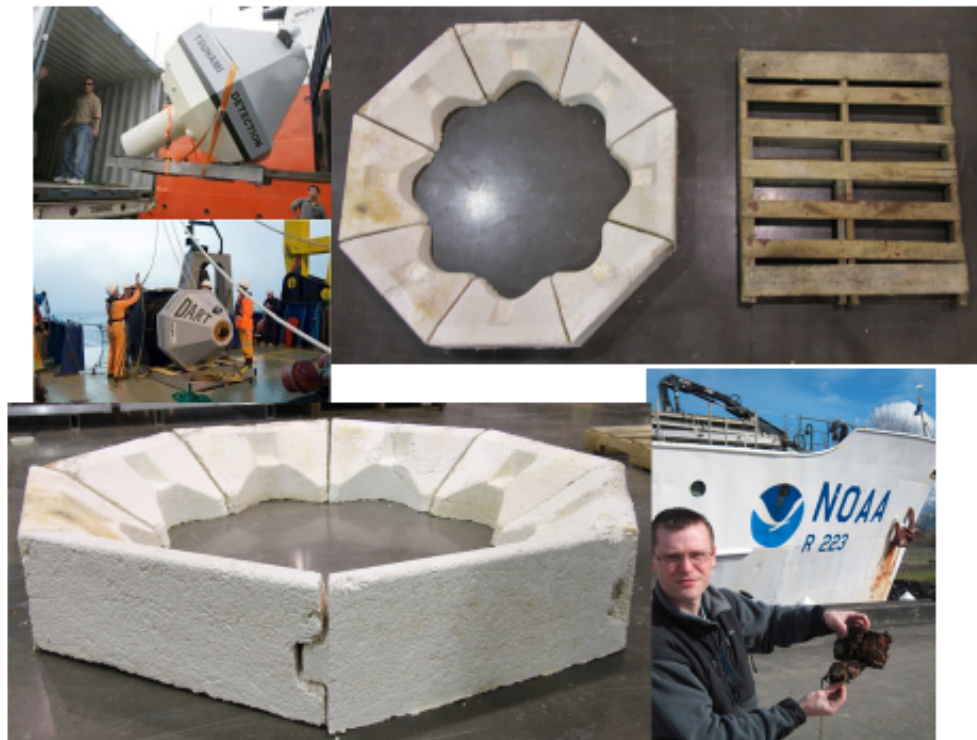
Figure 1. The myceliated composite developed as a one-use-cushion for the deployment of tsunami buoys.
