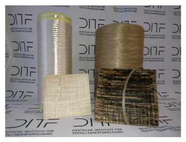
PureCell - pure composite material made from cellulosic tire cord fibers (left) and from natural fibers (right) by DITF Denkendorf
