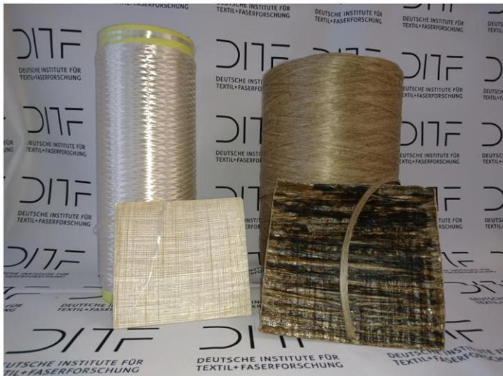
*PureCell - pure composite material made from cellulosic tire cord fibers (left) and from natural fibers (right) by DITF Denkendorf*
